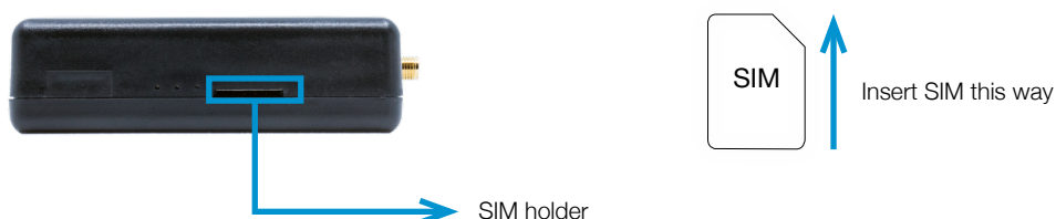
Figure 22. ZETA-NLP and ZETA-NSP - SIM holder
